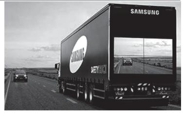
GREAT SAFETY IDEA - High accident statistics is the motivation for Samsung's latest development of what could be 'a road safety revolution'; the Safety Truck. The truck has a wireless camera in front which is connected to a video wall with four large monitors at the back of the truck.
